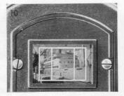
that the eyepiece (7) is not pushed forward, lest the picture field be distorted. Also take care that the horizontal and vertical lines of the subject run parallel to the edges of the finder.
