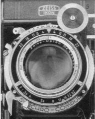
time is set before or after cocking the shutter. With the  $^{1}/_{500}$  sec. setting, the exposure time must be set before the shutter is wound.
